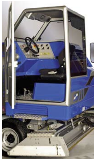
Fig. 2: The vehicle uses two CAN networks, one for the engine and one for the electric machinery
