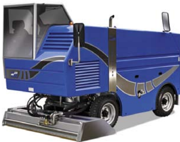
Fig. 1: The WM Evolution ice resurfacing machine is based on a CAN control system
