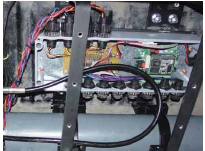
One of many computers in the vehicle, the H1ghlander's active suspension computer modifies the fluid level in the struts to keep the vehicle level and stable.
