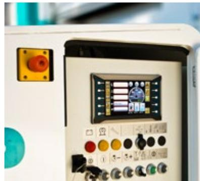
The operator interface has a powerful built-in display controller and is perfectly suited for the harsh conditions in off-highway vehicles due to the aluminium front. It is designed to become the central operator interface in mobile equipment such as mobile cranes, excavators or large drilling machines, like the Casagrande XP series.
